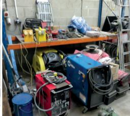
**WELDING:** MILLER Migmatic 300 Mig Welder; TELWIN Bimax Mig Welder; THUNDER 150GP Invertor Tig Welder & THERMAL DYNAMIC Cutmaster 38 Plasma Cutter.
